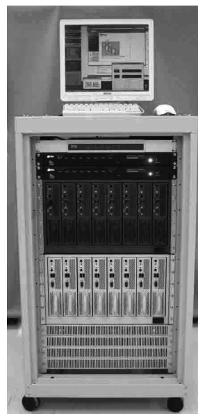
●図-5 汎用 20 U ラックへの搭載例● (Fig.5-Example of mounting blades into a general-purpose 20U rack)
